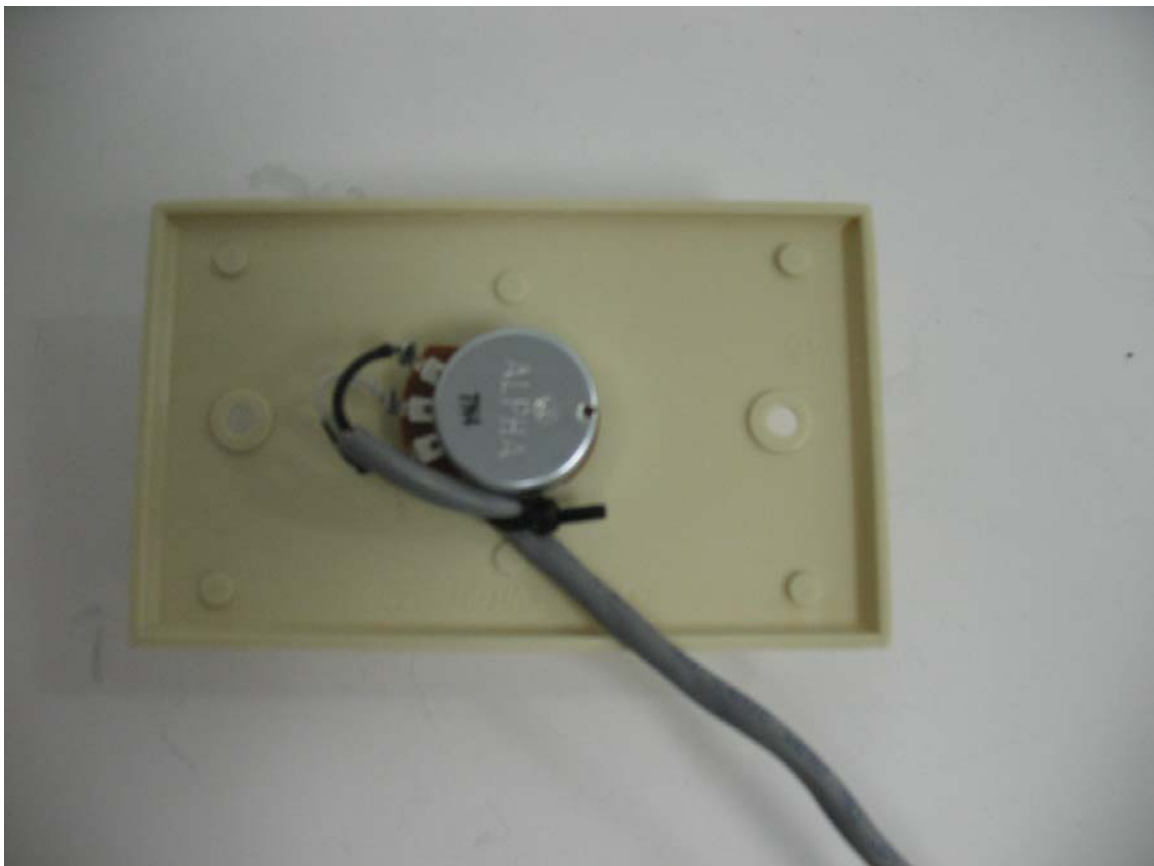
Fig. 3 The wiring of the Potentiometer.
